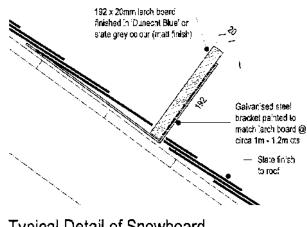
Typical Detail of Snowboard & Bracket Installation 1:2
