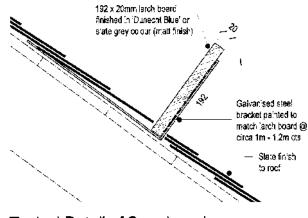
Typical Detail of Snowboard & Bracket Installation 1:2
